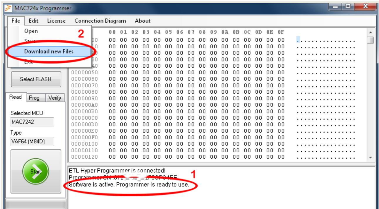
Figure 22 Download the new Files procedure
