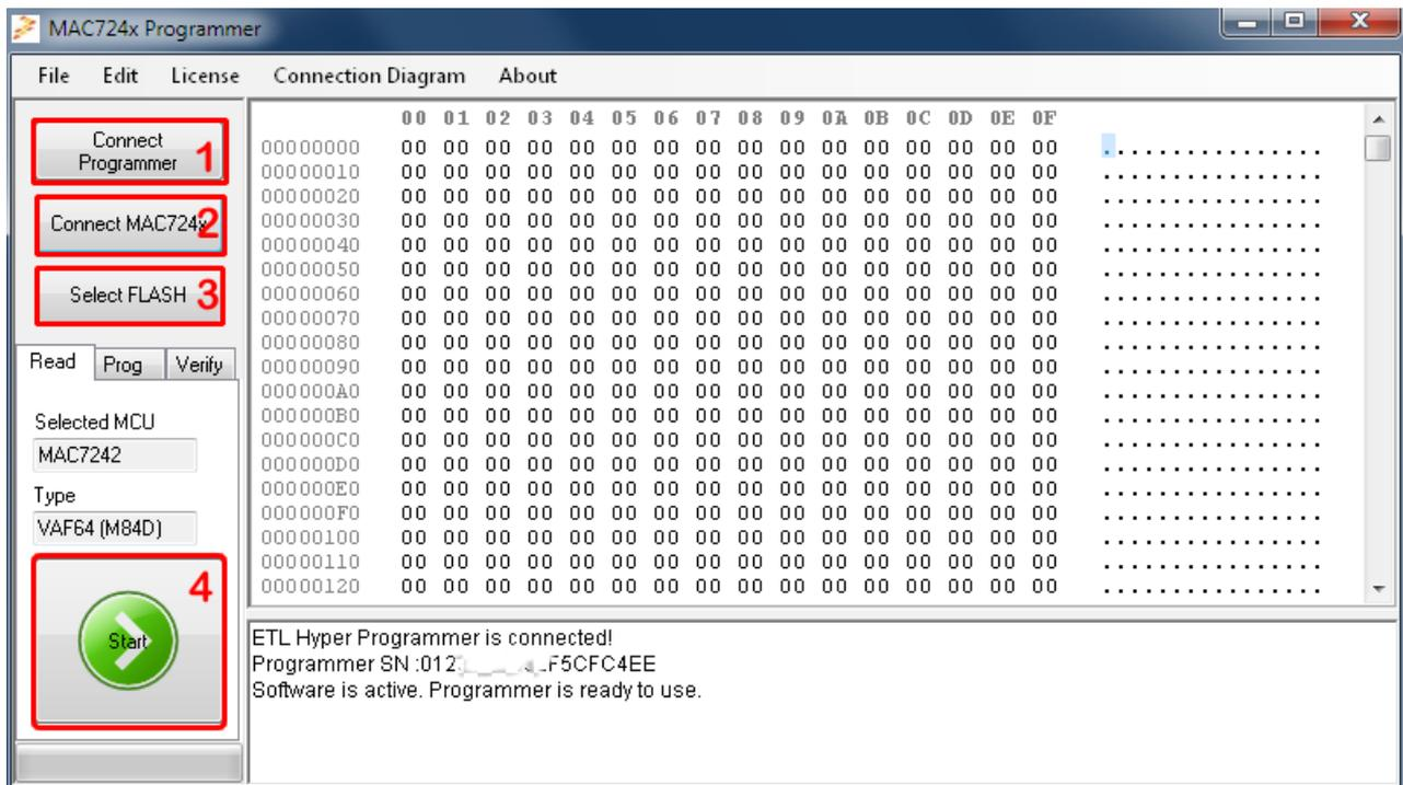
Figure 23 **MAC724x-Programmer** reading sequence.
