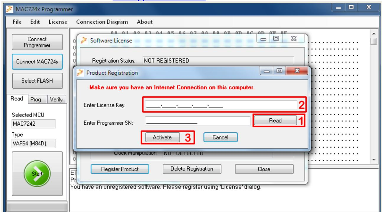
Figure 20 MAC724x-Programmer software activation
