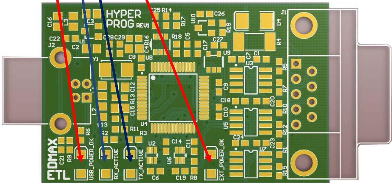
Figure 1. The ETL HYPER PROG board layout
