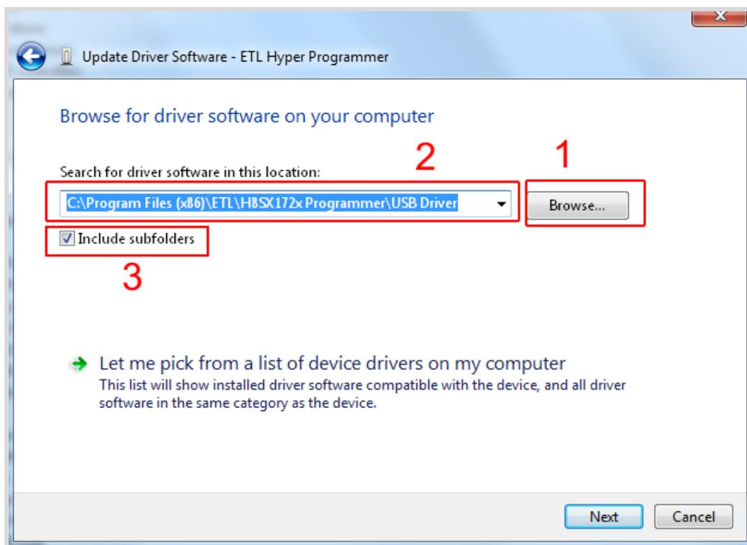
Figure 6. Update Driver Software - "ETL Hyper Programmer"
