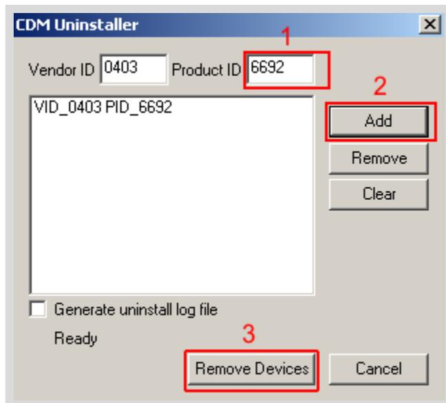
Figure 18 The Drivers uninstall by CDM Uninstaller software
